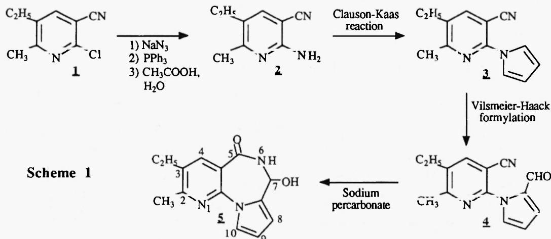
The continuation of this synthetic route uses two classical methods: the Clauson-Kaas reaction (6) with 4-chloropyridine hydrochloride as a catalyst, providing the pyrrolyl derivative **3** (75%), then
