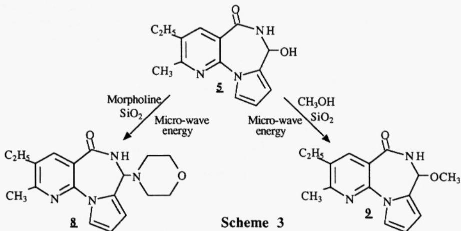
The hydroxydiazepine **5** and an excess of morpholine or methanol is dissolved in acetonitrile. The mixture is then refluxed in a microwave oven in the presence of silicagel as a catalyst and the reaction is monitored by thin layer chromatography. This procedure furnishes the amine **8** (55%) and the ether **9** (67%).
